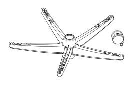
Place the 5 star base upside down and install the casters by firmly pushing the metal stem into the appropriate pocket until fully seated.
