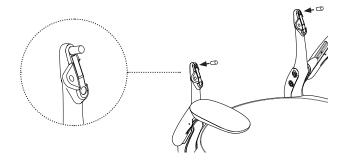
Install the hard foam parts on both sides of the seat frame.
